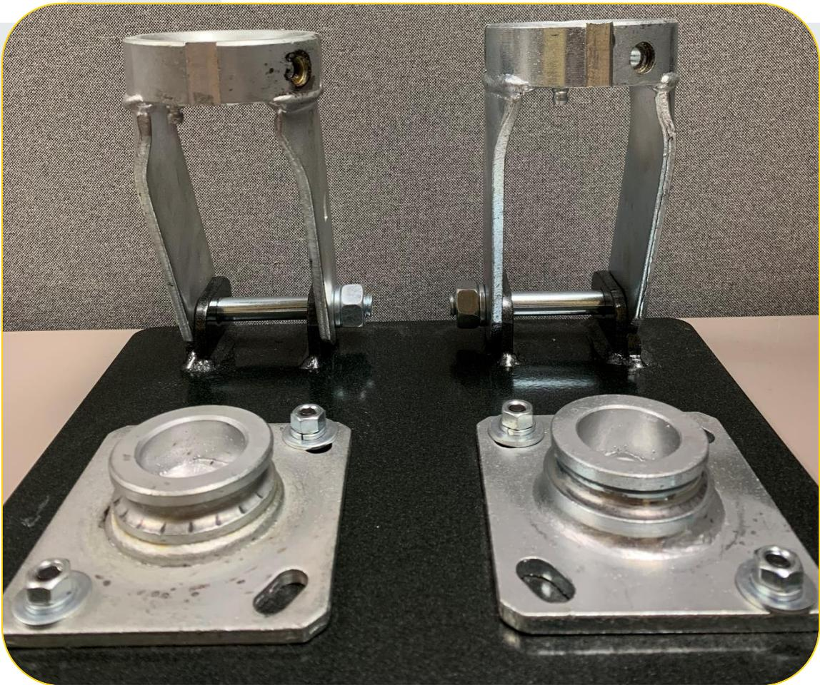
Images compare the non-heat treated caster (left) and the heat treated caster (right)
