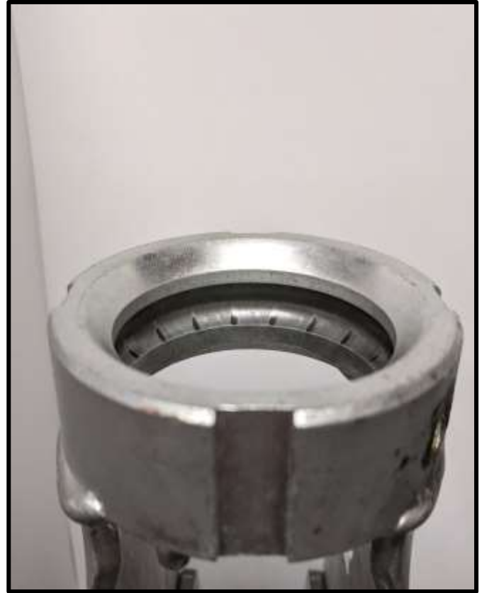
Competitor Equivalent Non-Heat Treated Raceway after 2 Hour Obstacle Test
