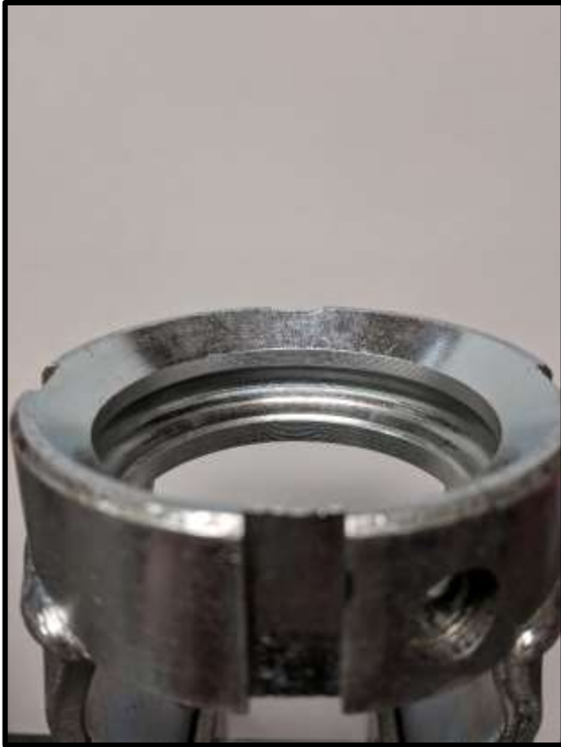
RWM 65 Series Heat Treated Raceway after 2 Hour Obstacle Test
